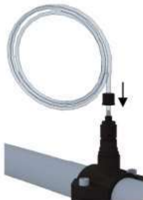
Thread the PE tubing through the cap and push it onto the valve cone.
