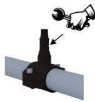
Tighten the injection valve onto the union
