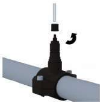
Loosen the injection valve nut.
