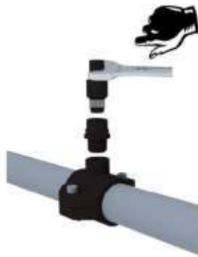
Screw the union onto the saddle clamp
